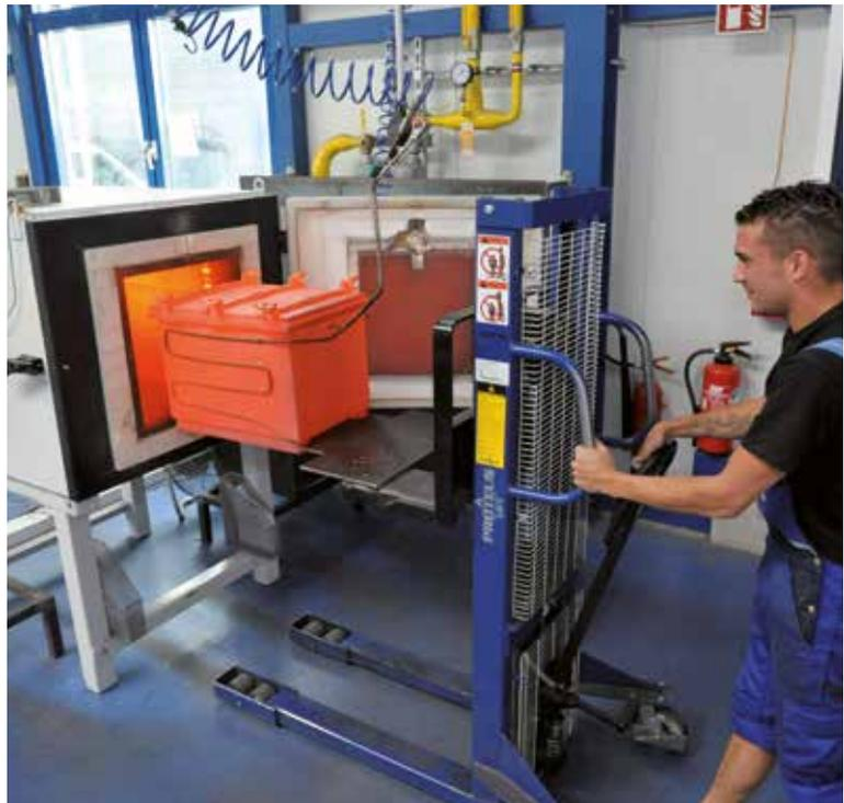
Air-circulation chamber furnace with gas box and charging stacker
