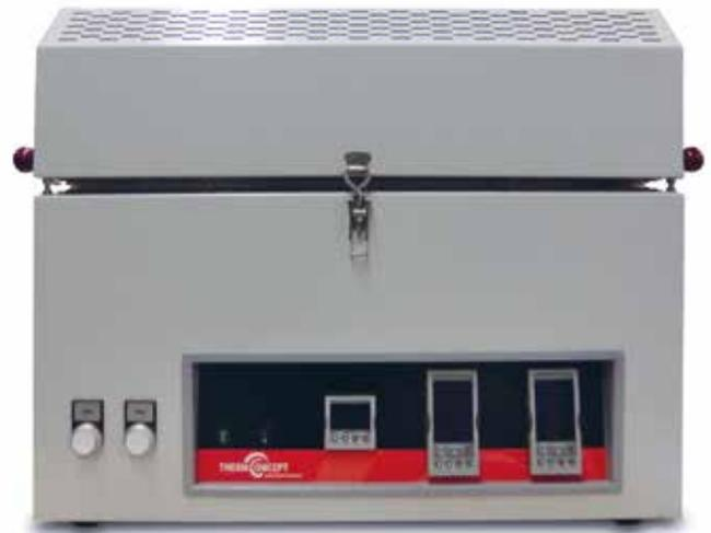
Split tube furnace with 2 independent control zones for thermal transport
